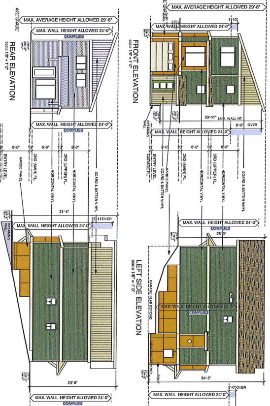
TYPE 2 (UNIT#8, 9 & 10) SHOWN IN COLOUR SCHEME F (UNIT 9) Average Height is 29'-5" Maximum is 29'-6" (1'-9" Over) Max. Wall Height is 23'-0" (Varies complies to 8'-9" over)
